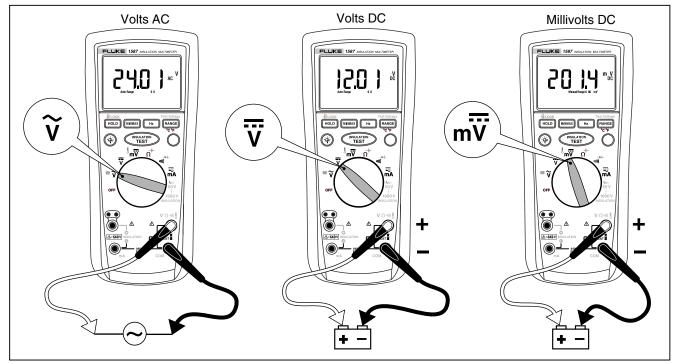
Figure 6. Measuring AC and DC Voltage
