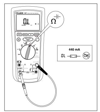
Figure 15. Testing the Fuse
