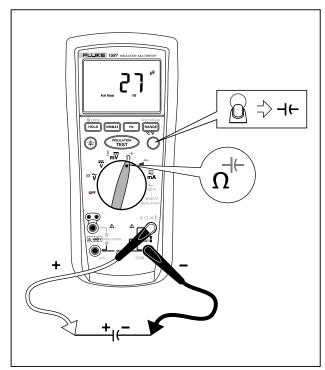
Figure 9. Measuring Capacitance
