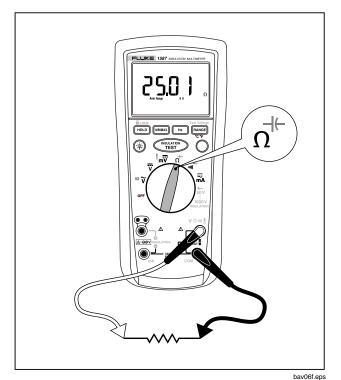
Figure 8. Measuring Resistance
