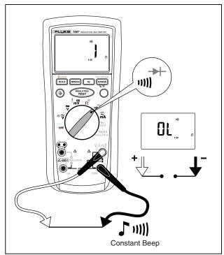
Figure 10. Testing for Continuity
