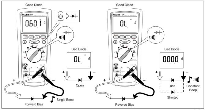
Figure 11. Testing Diodes
