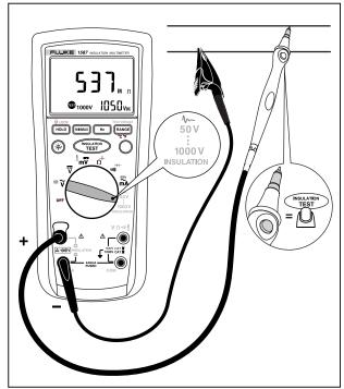
Figure 13. Testing Insulation
