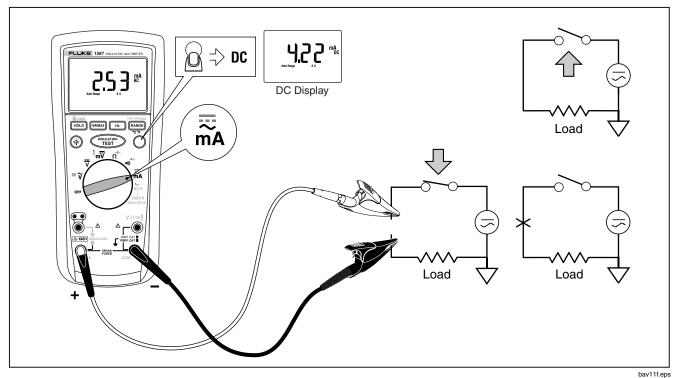
Figure 12. Measuring AC or DC Current
