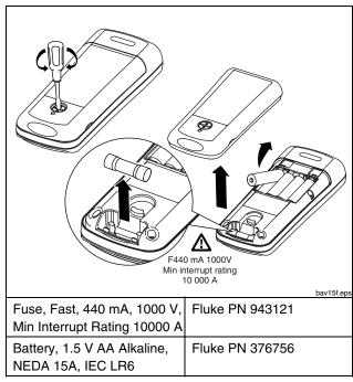
Figure 16. Replacing the Fuse and Battery
