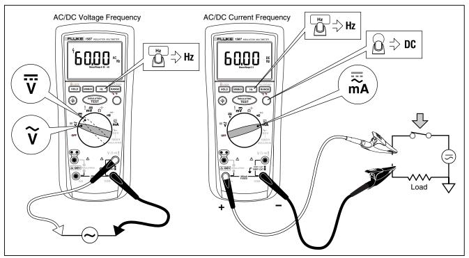
Figure 14. Measuring Frequency
