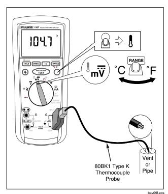
Figure 7. Measuring Temperature
